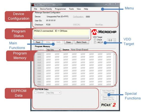
5.4 If the program status box shows "PICkit 2 not found, ...", then user is required to replug the iCP01 and to click [**Tools**] -> [**Check Communication**] for connecting the iCP01 with PICkit software.
