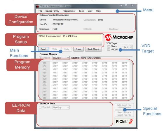
5.4 If the program status box shows "PICkit 2 not found, ...", then user is required to replug the iCP02 and to click [Tools] -> [Check Communication] for connecting the iCP02 with PICkit software.
